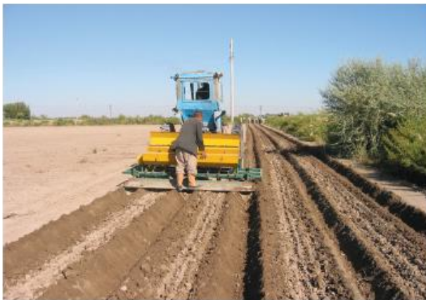
Figure 8: An Indian no till bed planter. Source: http://www.fao.org/ag/ca/doc/CA_UZB_WP2.pdf
