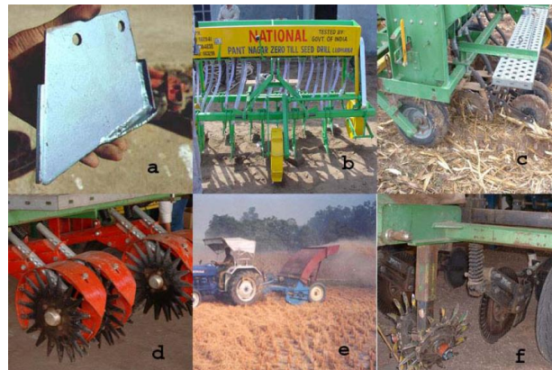
Figure 6: Various equipment for planting wheat no-till. (a) inverted-t coulters; (b) indian no-tillage drill using inverted t; (c) disk type planter; (d) star-wheel punch planter (e) "happy planter", which picks up straw and blows it behind the seeder; (f) disk planter. Source: http://www.ecaf.org/index.php?option=com_content&task=view&id=93&Itemid=64
