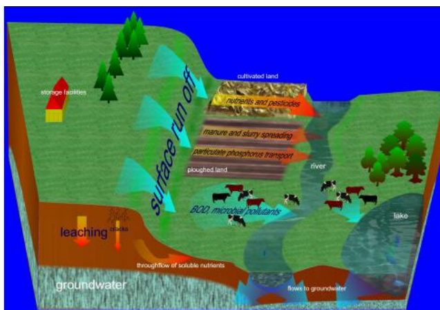
Figure 1: Main pathways by which agricultural pollutants can reach surface and groundwater. Source: http://www.ars.usda.gov/is/np/Phos&Euro2/agphoseuro2ed.pdf
